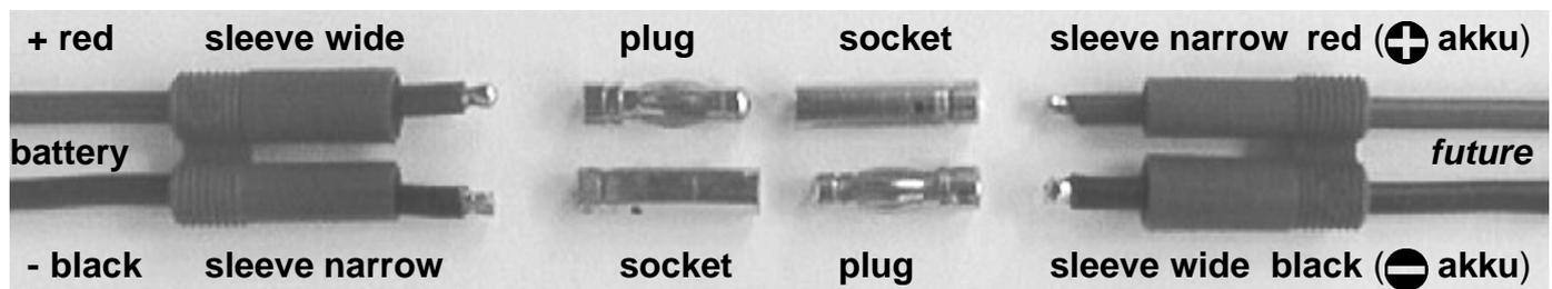
Fit the connectors in the order shown above; the contacts are pressed in as follows:
