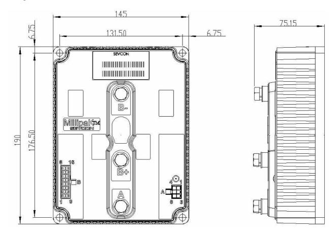
Maximum terminal torque: M8 terminals – 10NM
