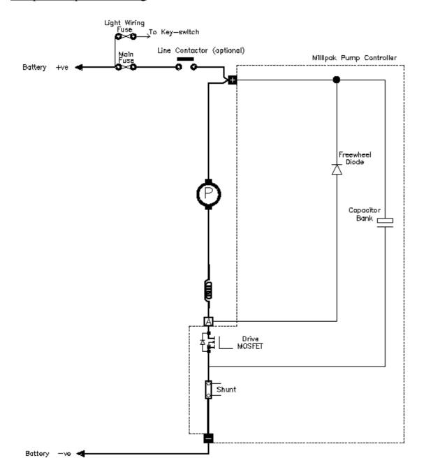
NOTE: The Pump battery positive power terminal may be wired directly to the battery positive (via a suitable fuse) or via a line contactor if used in a Traction / Pump system.
