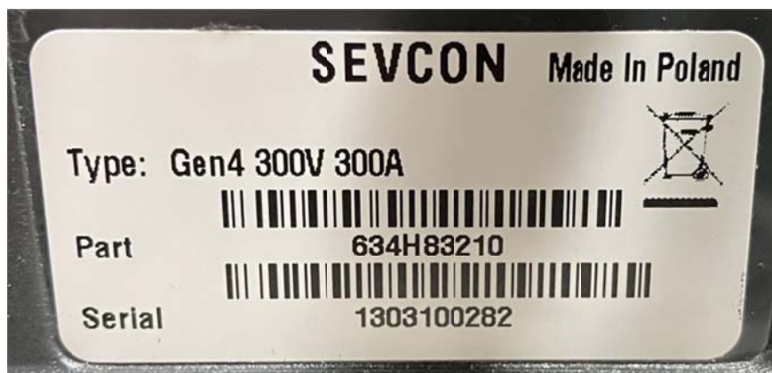
Fig. 5. The SEVCON GEN4 size 8 controller 634H83210 [2].
