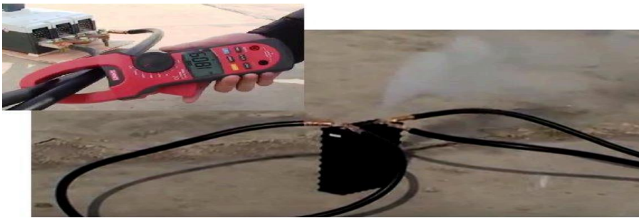
A short-circuit test on a fully charged Sinopoly cell. The current is exceeding 1800A as the cell is venting profusely.
