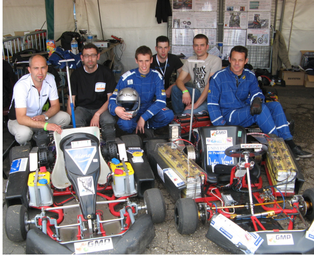
Fig 5 : 2 motors go-karts with normal rated power 28kW. 48V lead-acid(left) and 96V LiPo (right) e-kart challenge 2011.
