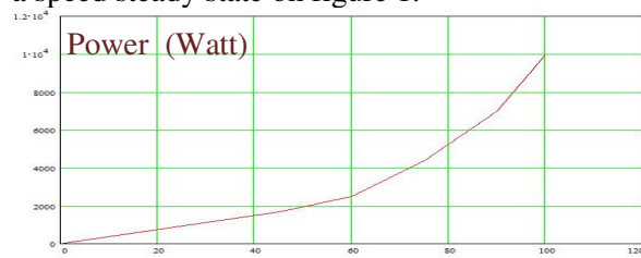
Figure 1: Motive power vs speed [M=200\text{kg}, f_a=0,01 \text{ N}/(\text{m}\cdot\text{s}^{-1})^2]
