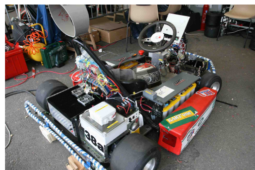
Figure 12. An embedded controller on a go-kart for wireless communications
